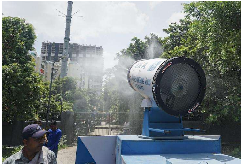
Image: Anti-Smog Gun in Delhi. An Anti-Smog Gun is a device that spews fine nebulized water droplets into the atmosphere so that the smallest dust and polluted particles are absorbed. (Image Source: PTI)
